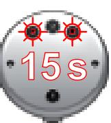
Change filter (see page 22). The alarm is first displayed when the machine is switched on and repeated every hour.
