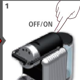
1 If alarm is repeated after switch ON/OFF several times: Descale machine (see page 18-19).
